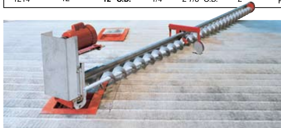
Commercial Klean Sweeps may also be used with U-Trough or Drag Conveyors.
