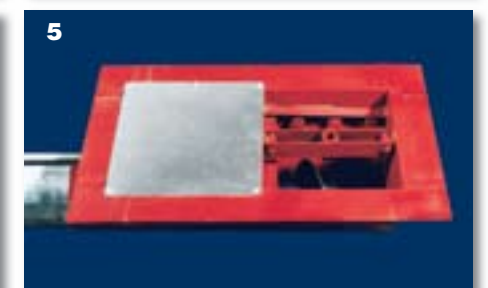
Photo 4 & 5: Bin wells have 1/4" plate steel gates supported by rollers; Gates slide into chambers protected from grain weight. May be used under suspended floor, in a trench or cast in concrete.
