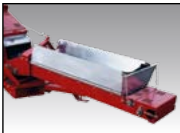
The Squeeze Belt® Conveyor features an Intake Transfer Hopper with independent adjustable hopper side panels. The hopper features a length of 70" with a width of 42" and a minimum hopper height of 10".
