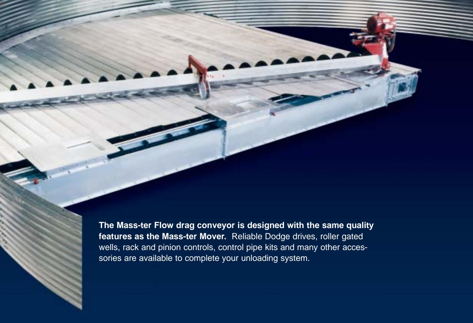
The Mass-ter Flow drag conveyor is designed with the same quality features as the Mass-ter Mover. Reliable Dodge drives, roller gated wells, rack and pinion controls, control pipe kits and many other accessories are available to complete your unloading system.
