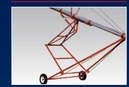
Available on 8" and 10", models in the 52', 62' and 72' lengths. Incorporates a hydraulic cylinder for raising and lowering, eliminating the need for hand cranking.
