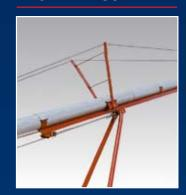
Steel rollers are used on a double angle-iron track for smoother operation.
