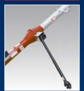
The PTO drive is fully shielded and conveniently located for safe operation. The PTO can be positioned to operate from either the left or right side of the auger. A lockable carrier for transport is standard.
